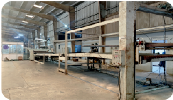
5 Ply Corrugation Machine Capacity : 2000 Ply Per Hour
