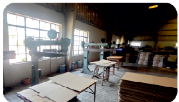
Corrugated Board Stapling Machine
