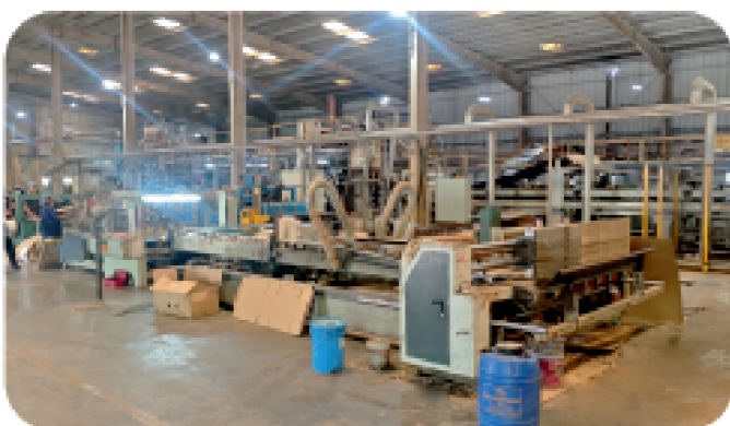
Corrugated Board Gluing Machine Capacity : 2000 Ply Per Hour
