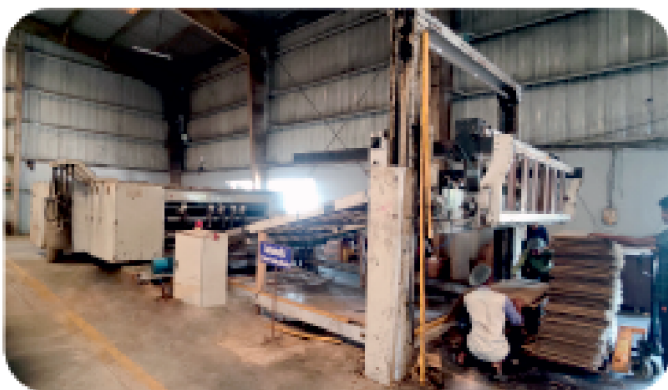
Automatic Two Colour Printing Machine Capacity : 12000 Boards Per Hour
