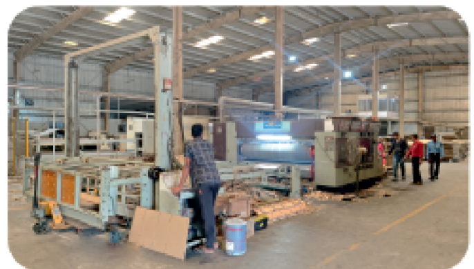
Automatic Two Colour Printer / Slotter Cum Rotary Die Cutter Machine
